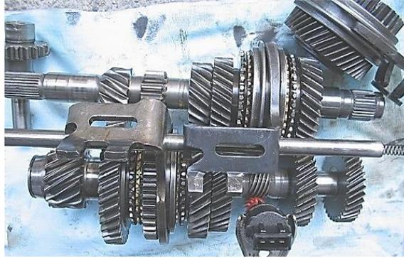
Figure 2-56: a typical example of gears - a five-speed + reverse gearbox from the Volkswagen Golf 1600cc (2009)
